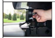
**Step 1.** Begin by removing the bulb and socket assembly from the marker light. Twist the socket up and away from the vehicle until it loosens.
