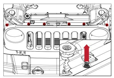
2. Pull bottom of grille away from vehicle to disengage metal clips on bottom rear of grille. Remove factory grille from vehicle.
