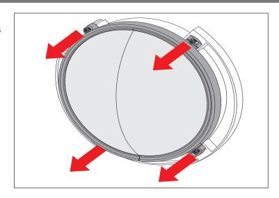
5. Using removed OE screws, install Elite Headlight Guard using T15 screwdriver or socket.
