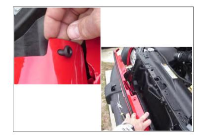
3. If desired the grille can be removed by disconnecting the two front turn signal bulbs and gently popping the grille from its lower retainer clips.
