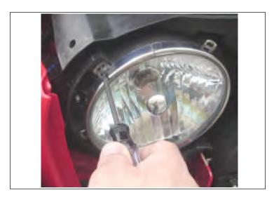
5. With ring removed place new Euro Guard retainer ring over lamp, aligning the tabs as shown.
