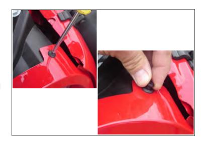
2. With the screws removed pop out the black retainer clip. Gently pull the grille forward.
