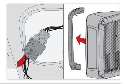
3. Encase tail light inside Housing and Guard using M5 Screws.
