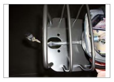
8. Re-connect the wiring connectors and guide the wiring back into the body.
