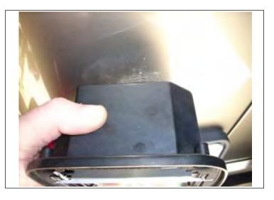
5. Carefully pull the tail light wiring through the hole. Guide the connector through the hole.
