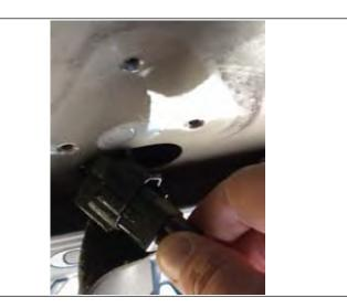
9. Reinstall the tail light assembly and Euro Tail Light Guard to the original mounting holes using the new bolts provided.
