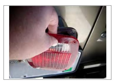
3. Remove the 3 tail light assembly retaining bolts.
