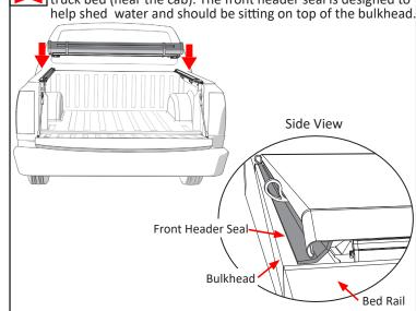
To connect the cover assembly (C) to the side rails (A & B), slide the right and left header guides into the locked position. A clicking sound will indicate a secure attachment.
