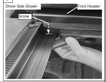
7 If socket doesn't fit on the fastener nut due to interference with the metal gusset, then reposition the rail rearward slightly
