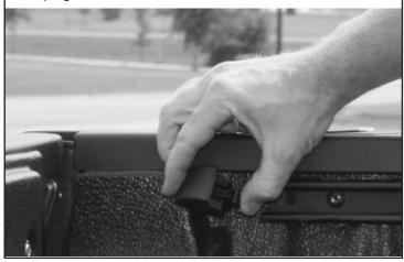
Remove tie downs: If tie downs are installed remove them from the cargo rail.
