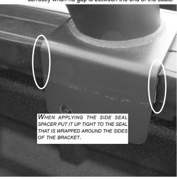
**STEP 6:** Cut the side seal spacer at the rear of the truck bed as indicated below.
