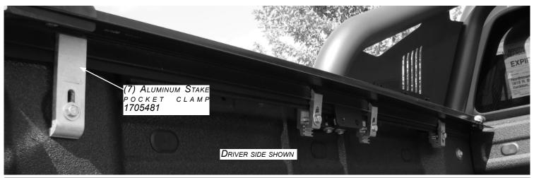
STEP 9: Install a shim for each clamp underneath the bed cap in the location that clamp will be mounted.
