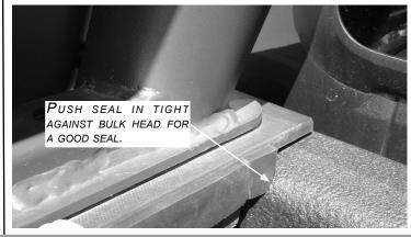
STEP 5: The side seal spacer needs to be cut on both sides of the sport bar bracket as indicated below. The seal is installed correctly when no gap is between the end of the seals.
