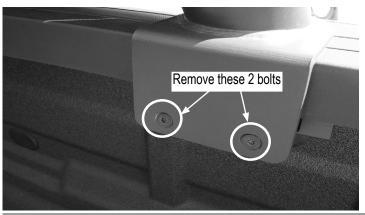
STEP 2: Using T30 Torx wrench loosen both screws located in the two holes located below.
