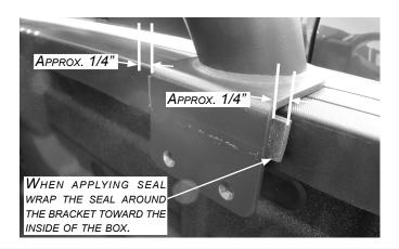
**STEP 4:** Apply side seal spacer along bed rail flush with the top of the bed cap.
