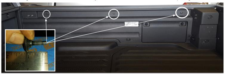
**STEP 2:** Mount brackets on driver and passenger sides using the factory installed M6 Shoulder bolts. Leave finger tight for now.
