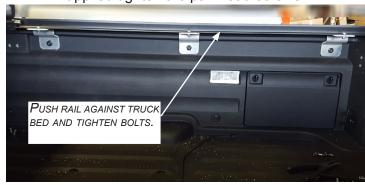
STEP 6: Tighten all fasteners. Repeat steps 1-5 on driver's side.
