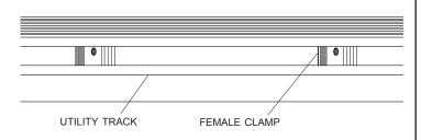
STEP 2: Evenly space and fasten male clamps loosely to female clamps with 3/8" x 1 1/2" cap screws.
