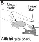
hook tailgate header into header stops on both sides of vehicle.
