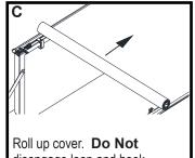
disengage loop and hook fasteners prior to rolling up cover.
