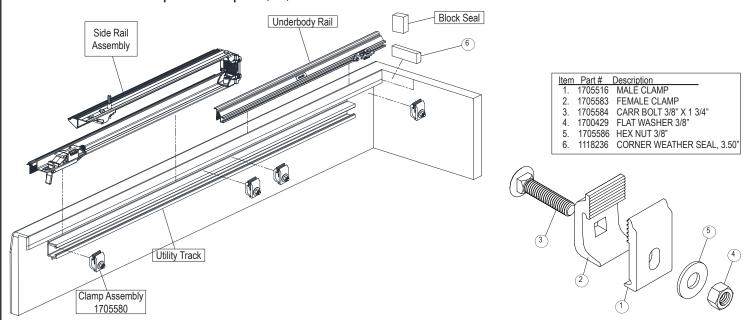
Install Underbody Rails: Apply bulkhead weather seal to bulkhead. Make a mark 30-1/4" back from bulkhead seal. Place block seal in corner against bulkhead seal. Seat the underbody rail against the top and inside of the bed rail and slide forward into block seal until the rear of the rail is flush with the mark you made. Clamp tightly using clamp in front of the utility track and clamp above the utility track.
