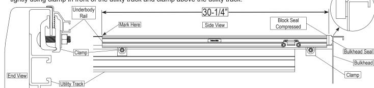
Install Underbody Rails: With the front part folded over, place the front end of the rear side rail flush to the rear of the underbody rail. Seat the rear side rail against the top and inside of the bed rail making sure the side rail seal is compressed. Clamp to pickup using one clamp behind the utility rail, and one clamp above the utility rail. Repeat steps 1-2 on Passenger Side.
