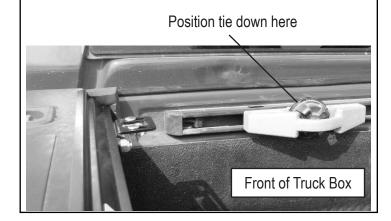
Install the underbody rails: The underbody rails are marked driver and passenger side. Clamp the underbody rails to the trucks bed rail. The underbody rails will be placed in front of the rear rail and right above the trucks cargo rail. Refer to step two in Deuce manual 1117648 for further positioning information.
