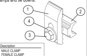
Install clamps in cargo rail as shown below: After clamps and tie down are installed replace the cargo rail end plugs. Leave clamps loose for now. Repeat steps 1 through 4 for the passenger side clamp installation.
