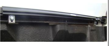
Install rear rail: With the underbody rails installed, position the rear rail along the inside edge of the truck box. Slide the rail forward so it is touching end to end with the underbody rail. Tighten clamps against the rail.
