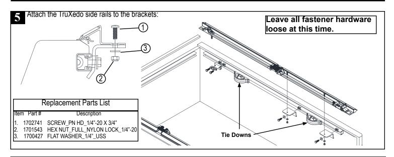
With the tailgate closed, center the side rail in the bed and position the center of the rear mounting bracket 11.25 inches from inside of tailgate. Tighten all top bracket fastener hardware. Then tighten all bottom bracket fastener hardware. This should pull the rail down to the truck bed. Follow the same procedure for the opposite side rail. Center spring latch base under striker pin and tighten both fasteners.
