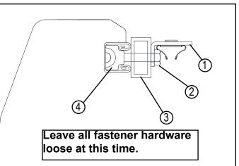
Install the side rail brackets into the cargo rails: Assemble the brackets as shown. Insert the assembled bracket into the cargo rail and slide to the middle. If cargo tie downs are going to be used slide one in on each side at this time. Insert the assembled bracket into the cargo rail and slide to the rear. Two brackets per side are required.
