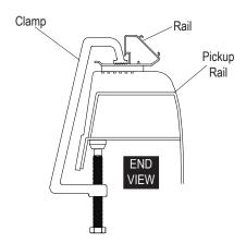
Do not attach clamps near one of the three holes in the underside of the pickup rail.
