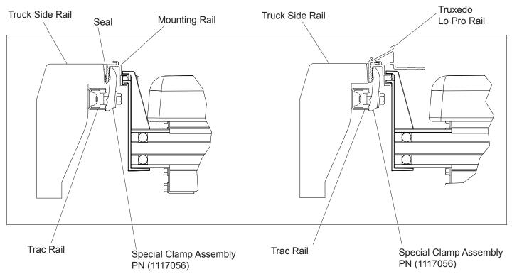
**Special Clamps:** Place clamps in the locations shown above. Driver side of mounting rail is shown. Follow the same assembly steps for the passenger side mounting rail. Refer to the owners manual for complete toolbox installation instructions
