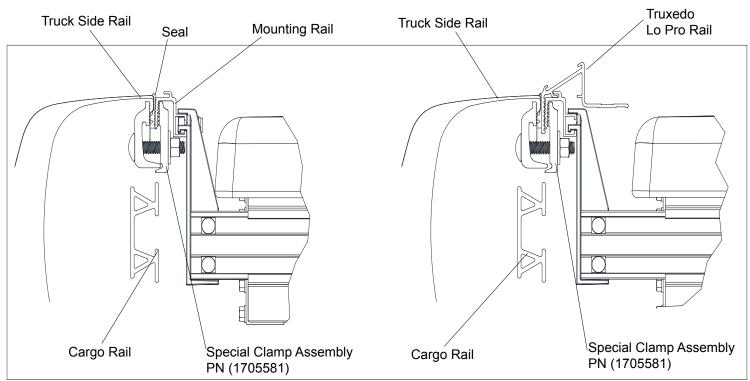
**Special Clamps:** Place clamps in the locations shown above. Driver side of mounting rail is shown. Follow the same assembly steps for the passenger side mounting rail. Refer to the owners manual for complete toolbox installation instructions
