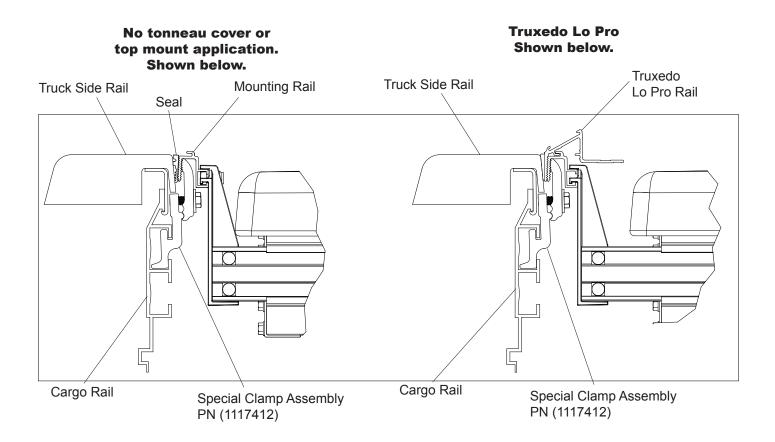
**Special Clamps:** Place clamps in the locations shown above. Driver side of mounting rail is shown. Follow the same assembly steps for the passenger side mounting rail. Refer to the owners manual for complete toolbox installation instructions
