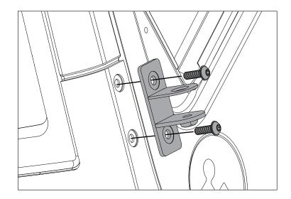
3. Attach Arm to Bushing. Using Thumb Screw, loosely install Bushing and Arm into Mounting Bracket.
