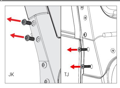
2. Using supplied hardware, install Mounting Bracket with welded nut facing down.
