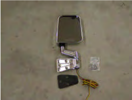
Figure 1. Kit includes one each of RIGHT and LEFT mirrors, all required wiring and hardware.
