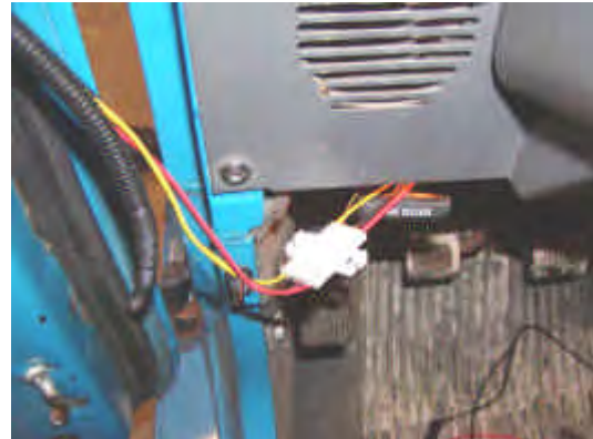
Figure 10. The final installation steps. Be sure wires correspond on both plugs. Place wiring in the loom. Tuck plugs behind dash. Test all light functions.
